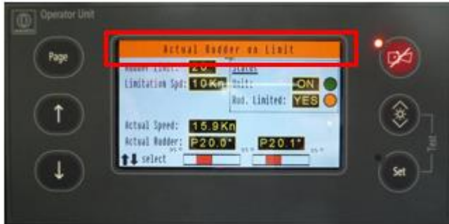
Figure 2-3 Alerts are presented at the message bar of the Rudder Limit Unit
